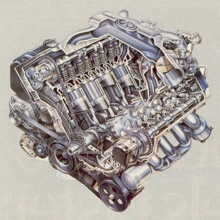
• An engine's performance is directly linked to its breathing efficiency. Increase the amount of air flowing into the cylinders and you increase the engine's specific output. This is the major benefit of switching from two valves per cylinder to four. But now Nissan and some other makers are enhancing their four-valve engines with variable-valve-timing systems. These VVT systems, such as the one found in the new Infiniti Q45, improve the performance of four-valve engines even further.
